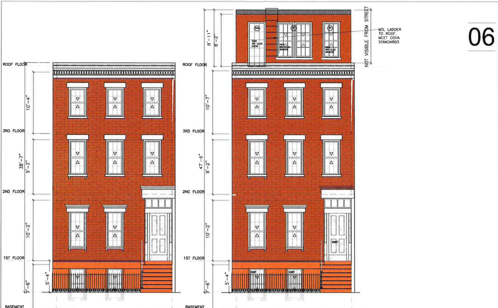
1 EXISTING FRONT ELEVATION @ 32th PERRY STREET 1/4" = 1'-0"
